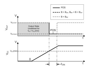
Figure 3: Power-On Timing Diagram
