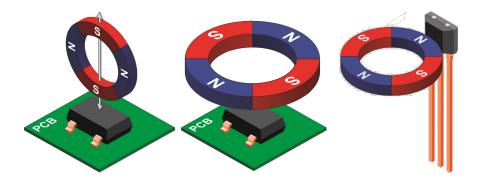
Figure 5: Sensing Configurations
