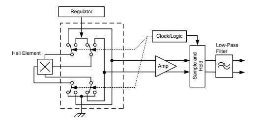
Figure 6: Model of Chopper Stabilization (Dynamic Offset Cancellation)
