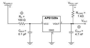
A R<sub>S</sub> and C<sub>OUT</sub> are recommended for maximum robustness in an automotive environment.
