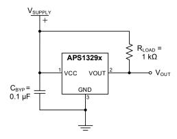
**Figure 1: Typical Application Circuit**
