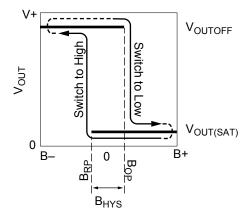
Figure 2: Switching Behavior of Latches
