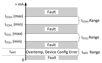
Figure 4: Interpreting I<sub>CC</sub> for System-Level Diagnostics
