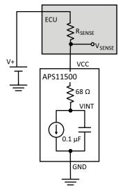
(D) High-Side Sensing (UC package)
