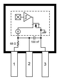
UC Package, 3-Pin SIP Pinout
