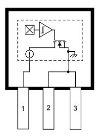
LH Package, 3-Pin SOT23W Pinout
