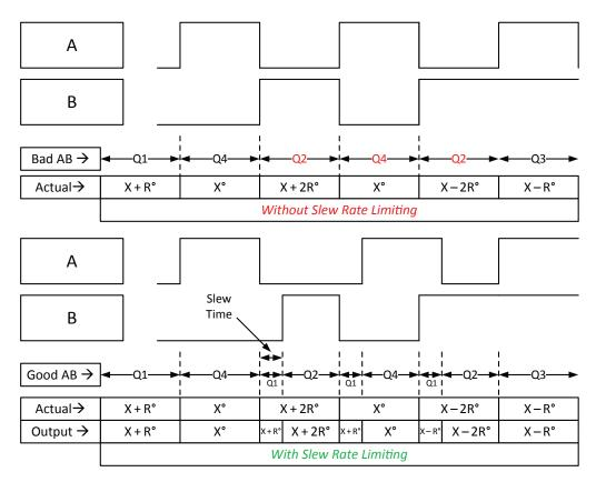
Figure 8: Slew Rate Limiting
