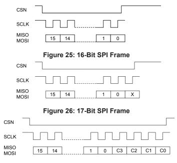
Figure 27: 20-Bit SPI Frame
