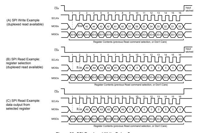
Figure 28: SPI Read and Write Pulse Sequences
