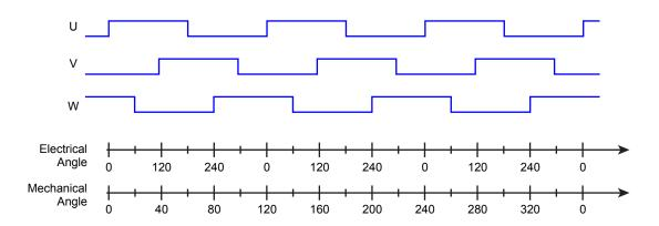
Figure 10: U, V, W Outputs for Three Pole-Pair BLDC Motor
