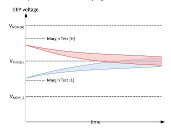
Figure 38: Example of failing programming voltages
