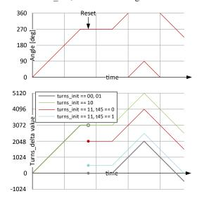
Figure 19: "turns\_delta" value at startup, depending on "turns\_init"
