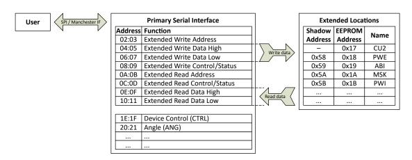
Figure 21: Serial Registers allow access to extended memory (EEPROM and Shadow)
