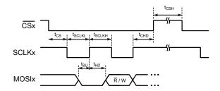
Figure 23: SPI Interface Timings Input
