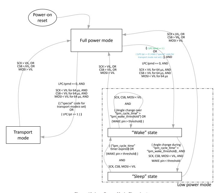
Figure 13: Low Power Mode Flowchart
