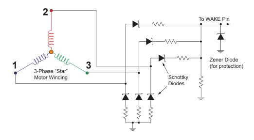
Figure 15: Sample Filtering Circuit
