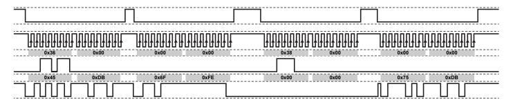
Figure 18: Read of a Negative turns\_delta Value
