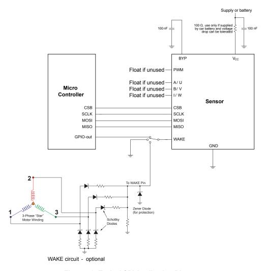
Figure 40: Typical SPI Application Diagram
