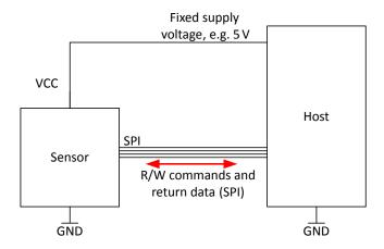
Figure 22: Programming Connections for SPI Interface
