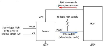
Figure 30: Manchester Interface Programming Setup
