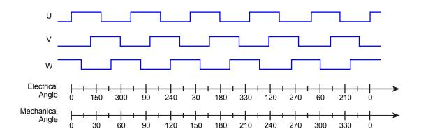
Figure 11: U, V, W Outputs for Five Pole-Pair BLDC Motor
