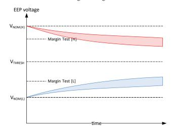
Figure 37: Example of passing programming voltages
