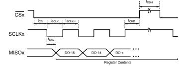
Figure 24: SPI Interface Timings Output
