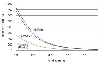
Figure 39: Magnetic Field versus Air Gap for a magnet 6 mm in diameter and 2.5 mm thick.
