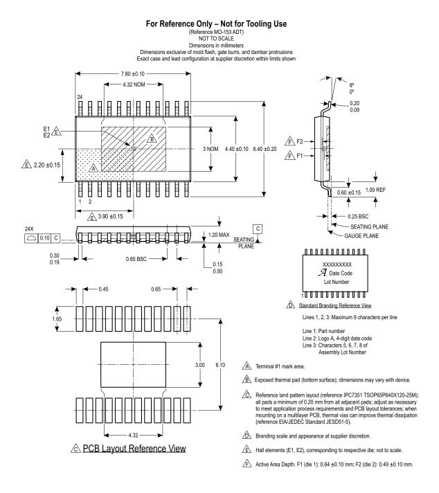
Figure 42: Package LP, 24-Pin TSSOP with Exposed Thermal Pad
