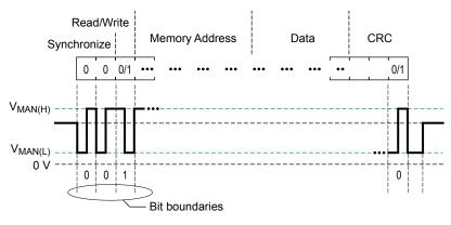
Figure 13: General Format for Serial Interface Commands
