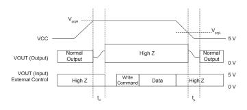
Figure 17: Write Volatile Memory
