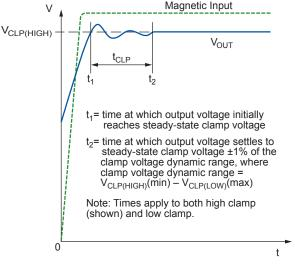
Figure 4: Delay to Clamp definition
