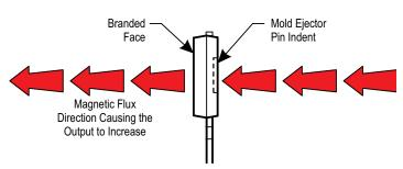
Figure 6: Magnetic Flux Polarity
