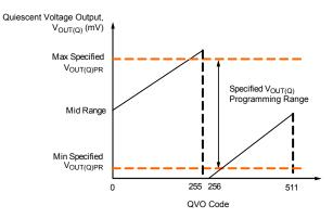
Figure 8: Device V<sub>OUT(Q)</sub> versus QVO Programmed Value
