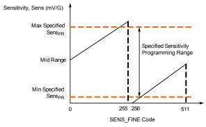
Figure 7: Device Sensitivity versus SENS\_FINE Programmed Value
