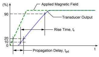
Figure 2: Propagation Delay and Rise Time Definitions
