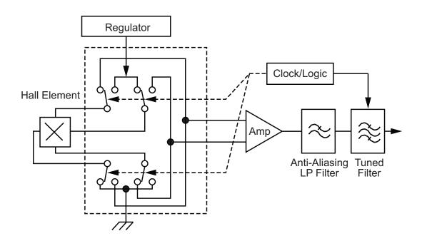
Figure 12: Concept of Chopper Stabilization
