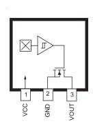
Package LH, 3-Pin SOT23W Pinout Diagram
