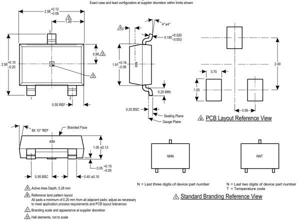
Figure 3: Package LH, 3-Pin SOT-23W
