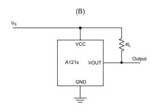
Figure 1: Switching Behavior of Latches
