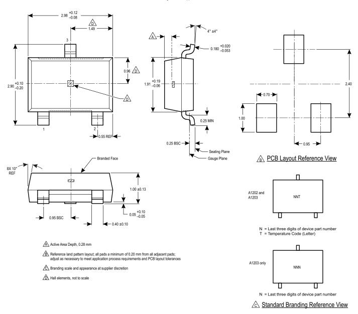
Figure 3: Package LH, 3-Pin (SOT-23W)
