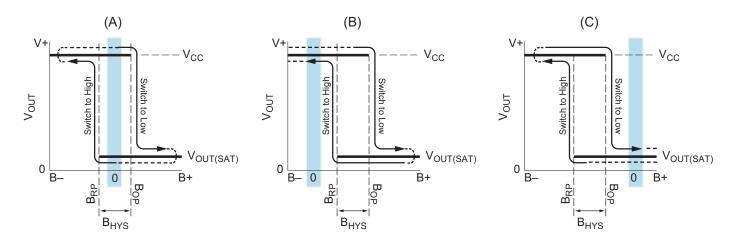
Figure 1: Bipolar Device Output Switching Modes
