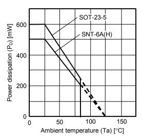
Figure 4 Power Dissipation of The Package (When Mounted on Board)
