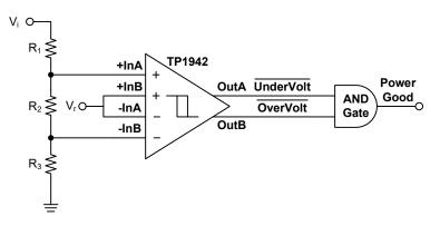
Figure 10. Windowed Comparator
