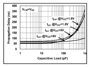
Propagation Delay Skew V.S. Capacitor Loading
