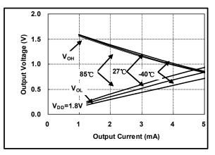
Output Voltage Headroom V.S. Output Current
