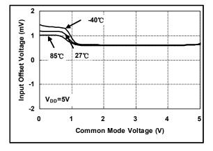
Input Offset Voltage V.S. Common Mode Voltage
