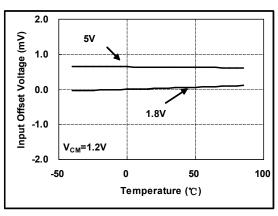
Input Offset Voltage V.S. Temperature
