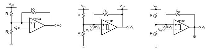
Figure 5. Inverting Configuration with Hysteresis
