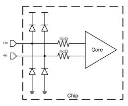
Figure 2. Equivalent Input Structure
