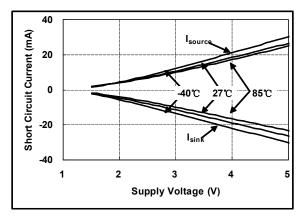
**Output Short Circuit Current V.S. Temperature**
