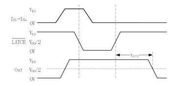
Figure 7. TP1941NU Timing Diagram with Latch Operator
