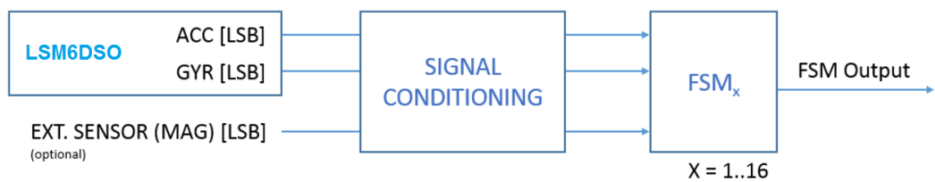
Figure 2. State machine in the LSM6DSO
