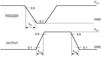
Figura 2. Switcing Waveforms
