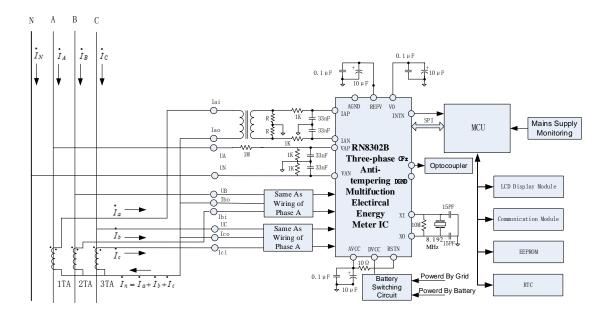
Figure 1-3 Typical Application Circuit Schematic of Three-phase Four-wire Meter
