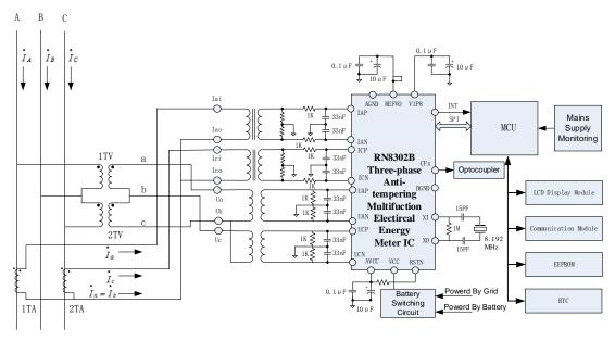
Figure 1-4 Typical Application Circuit Schematic of Three-phase Three-wire Meter
