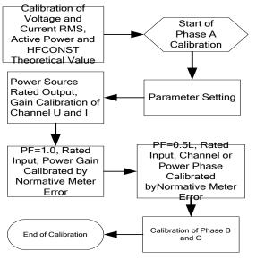
Figure 4-3 Pulse Method Calibration Flow
