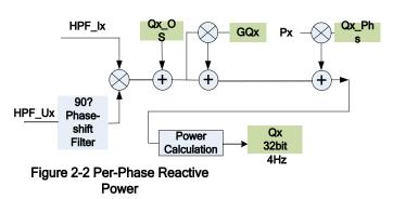
The RN8302B provides the total and fundamental per-phase reactive power and all-phase sum reactive power and provides the sign bit of the per-phase and the all-phase sum reactive power for the four quadrants judging. Furthermore, it provides the reactive power gain calibration,
