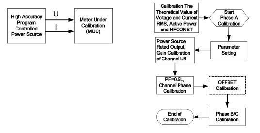
Figure4-1 Calibration Flow
