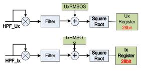
Figure 2-4 Voltage and Current RMS
