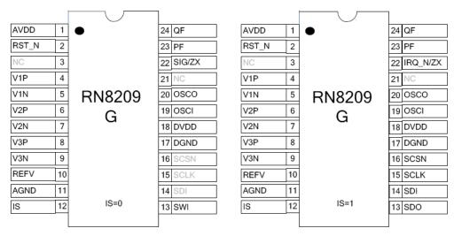
Figure 1-2 Pin Assignment
