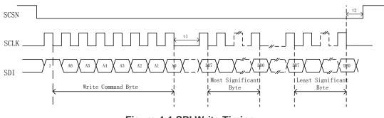
Figure 4-1 SPI Write Timing
