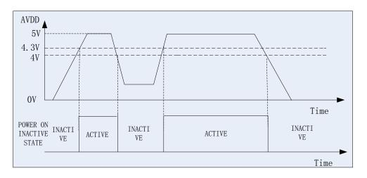
**Figure 2-1 Power Detection Features**
