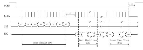
Figure 4-2 SPI Read Timing
