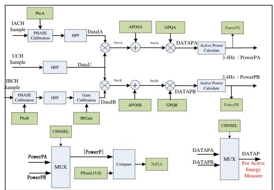
Figure 2-2 Active Power Diagram
