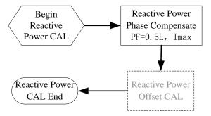
Figure 3-4 Reactive Calibration Flow
