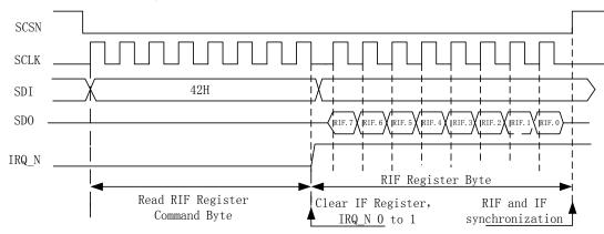
Figure 2-5 Timing Diagram for RIF Register Reading
