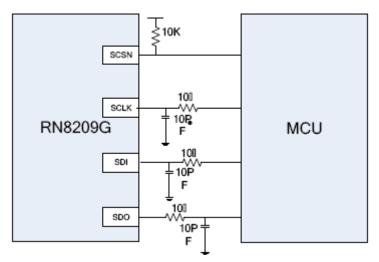
Figure 4-3 SPI Typical Connection
