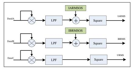
Figure 2-4 RMS Calculation Diagram
