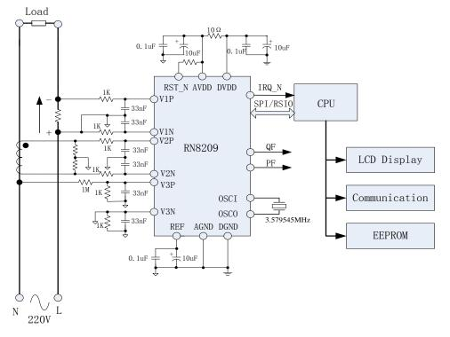
Figure 1-3 Typical Application of Single-phase Anti-tampering Meter
