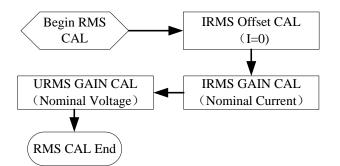
Figure 3-5 RMS Calibration Flow
