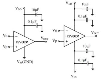
Figure 3. Amplifier with Bypass Capacitors
