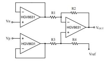
Figure 5. Instrumentation Amplifier
