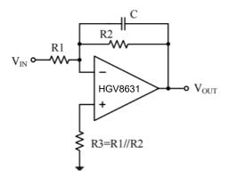
Figure6.LOW Pass Active Filter
