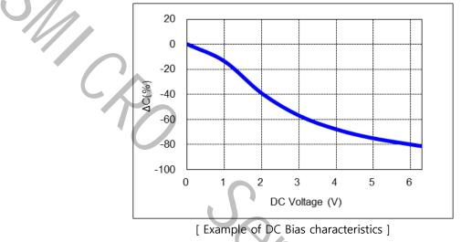
\* Sample : X5R 10uF, Rated voltage 6.3V
