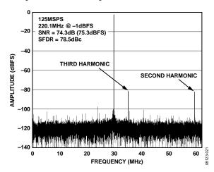
Figure 37. AD9268-125 Single-Tone FFT with  $f_{\text{IN}}$  = 220.1 MHz
