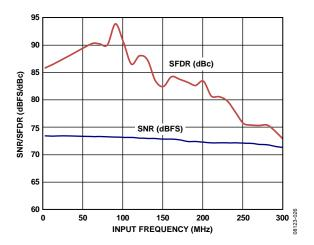
Figure 45. AD9268-125 Single-Tone SNR/SFDR vs. Input Frequency (flN) with 1 V p-p Full Scale
