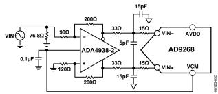
Figure 66. Differential Input Configuration Using the ADA4938-2
