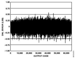
Figure 19. AD9268-80 DNL with  $f_{IN} = 9.7 \text{ MHz}$
