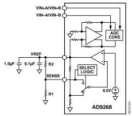
Figure 71. Programmable Reference Configuration
