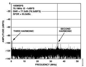
Figure 21. AD9268-105 Single-Tone FFT with  $f_{IN} = 70.1$  MHz
