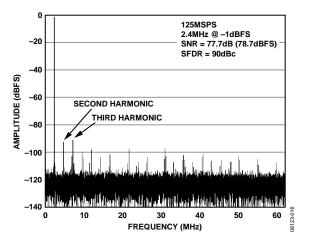
Figure 32. AD9268-125 Single-Tone FFT with  $f_{IN}$  = 2.4 MHz
