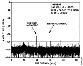
Figure 23. AD9268-105 Single-Tone FFT with  $f_{IN}$  = 200.3 MHz
