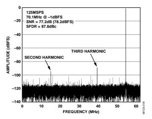
Figure 34. AD9268-125 Single-Tone FFT with  $f_{\rm IN}$  = 70.1 MHz
