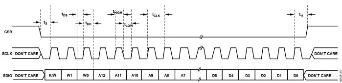
Figure 84. Serial Port Interface Timing Diagram
