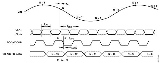
Figure 2. CMOS Default Output Mode Data Output Timing
