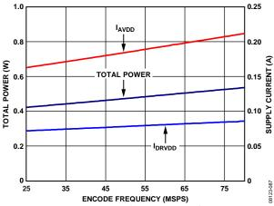
Figure 83. AD9268-80 Power and Current vs. Encode Frequency (LVDS
