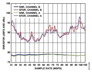
Figure 28. AD9268-105 Single-Tone SNR/SFDR vs. Sample Rate ( $f_s$ ) with  $f_{\rm IN}$  = 70.1 MHz
