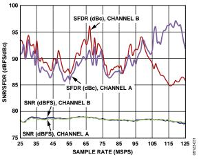
Figure 50. AD9268-125 Single-Tone SNR/SFDR vs. Sample Rate ( $f_s$ ) with  $f_{\rm IN}$  = 70.1 MHz
