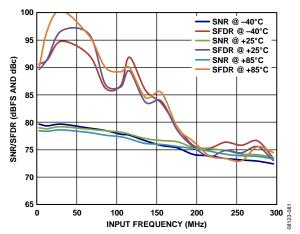
Figure 27. AD9268-105 Single-Tone SNR/SFDR vs. Input Frequency (f<sub>in</sub>) with 2 V p-p Full Scale
