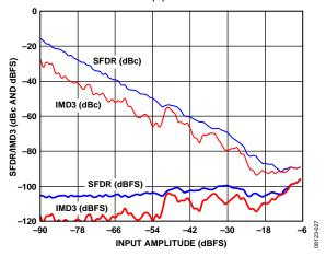
Figure 46. AD9268-125 Two-Tone SFDR/IMD3 vs. Input Amplitude ( $A_{\rm IN}$ ) with  $f_{\rm IN1}=29.1$  MHz,  $f_{\rm IN2}=32.1$  MHz,  $f_{\rm S}=125$  MSPS
