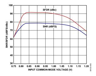
Figure 54. SNR/SFDR vs. Input Common Mode (VCM) with  $f_{\rm IN} = 30$  MHz
