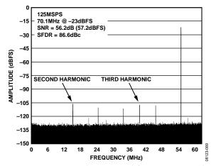
Figure 40. AD9268-125 Single-Tone FFT with  $f_{\rm IN}$  = 70.1 MHz @ -23 dBFS with Dither Enabled, 1M Sample
