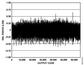
Figure 31. AD9268-105 DNL with  $f_{IN} = 9.7 \text{ MHz}$
