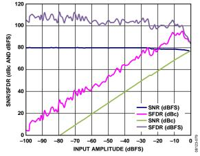
Figure 25. AD9268-105 Single-Tone SNR/SFDR vs. Input Amplitude ( $A_{\rm IN}$ ) with  $f_{\rm IN}$  = 98.12 MHz
