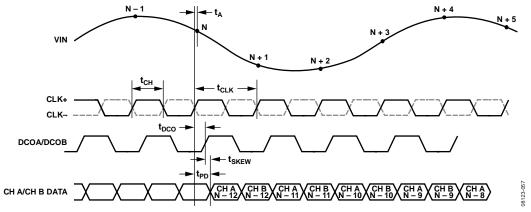
Figure 3. CMOS Interleaved Output Mode Data Output Timing
