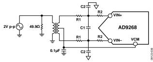
Figure 67. Differential Transformer-Coupled Configuration
