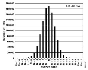
Figure 17. AD9268-80 Grounded Input Histogram
