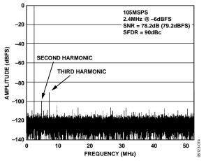
Figure 20. AD9268-105 Single-Tone FFT with  $f_{IN} = 2.4$  MHz
