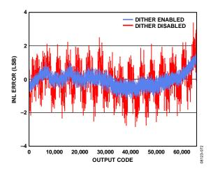
Figure 18. AD9268-80 INL with  $f_{IN} = 9.7 \text{ MHz}$
