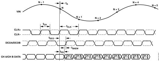
Figure 4. LVDS Mode Data Output Timing
