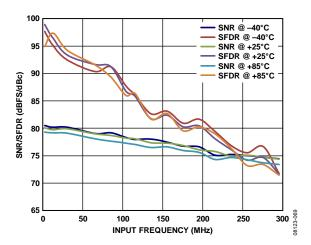
Figure 15. AD9268-80 Single-Tone SNR/SFDR vs. Input Frequency (f<sub>in</sub>) with 2 V p-p Full Scale
