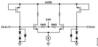
Figure 56. Equivalent Clock Input Circuit
