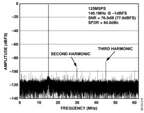
Figure 35. AD9268-125 Single-Tone FFT with  $f_{IN} = 140.1$  MHz
