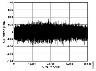
Figure 53. AD9268-125 DNL with  $f_{\text{IN}} = 9.7 \text{ MHz}$
