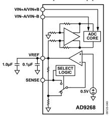
Figure 70. Internal Reference Configuration
