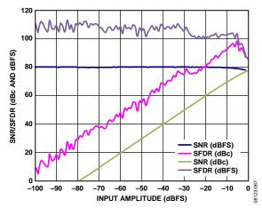
Figure 13. AD9268-80 Single-Tone SNR/SFDR vs. Input Amplitude (A<sub>IN</sub>) with  $f_{IN} = 98.12$  MHz
