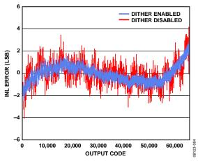
Figure 30. AD9268-105 INL with  $f_{IN} = 9.7 \text{ MHz}$
