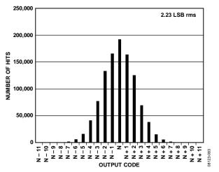
Figure 29. AD9268-105 Grounded Input Histogram
