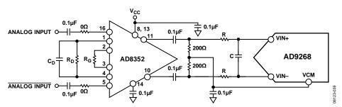
Figure 69. Differential Input Configuration Using the AD8352
