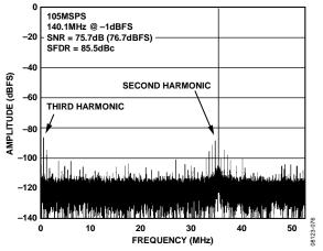
Figure 22. AD9268-105 Single-Tone FFT with  $f_{IN}$  = 140.1 MHz
