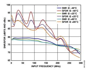
Figure 44. AD9268-125 Single-Tone SNR/SFDR vs. Input Frequency ( $f_{\rm IN}$ ) with 2 V p-p Full Scale
