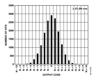
Figure 51. AD9268-125 Grounded Input Histogram
