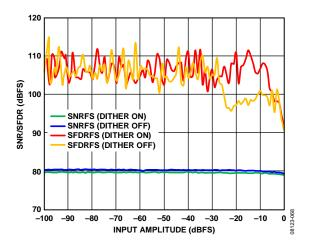
Figure 14. AD9268-80 Single-Tone SNR/SFDR vs. Input Amplitude ( $A_{IN}$ ) with  $f_{IN}$  = 30 MHz with and without Dither Enabled
