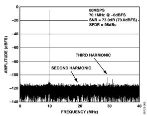
Figure 12. AD9268-80 Single-Tone FFT with  $f_{\rm IN}$  = 70.1 MHz with Dither Enabled
