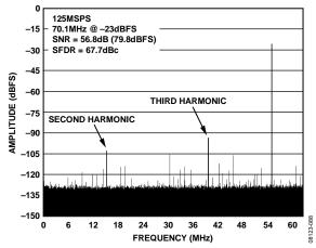
Figure 39. AD9268-125 Single-Tone FFT with  $f_{\rm IN}$  = 70.1 MHz @ -23 dBFS with Dither Disabled, 1M Sample
