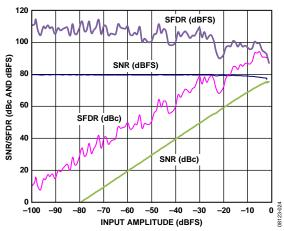
Figure 42. AD9268-125 Single-Tone SNR/SFDR vs. Input Amplitude ( $A_{IN}$ ) with  $f_{IN} = 98.12$  MHz
