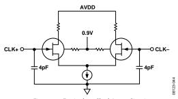
Figure 74. Equivalent Clock Input Circuit
