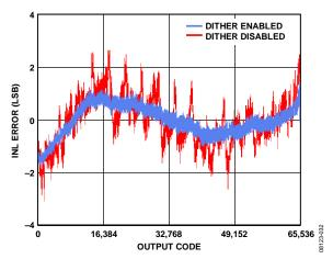
Figure 52. AD9268-125 INL with  $f_{\rm IN}$  = 9.7 MHz
