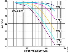
Figure 80. SNR vs. Input Frequency and Jitter
