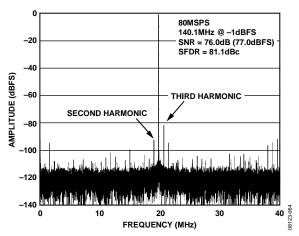
Figure 10. AD9268-80 Single-Tone FFT with  $f_{\text{IN}}$  = 140.1 MHz
