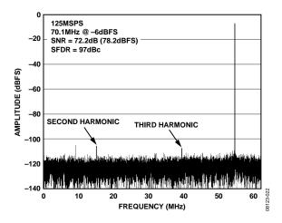
Figure 38. AD9268-125 Single-Tone FFT with  $f_{\rm IN}$  = 70.1 MHz @ -6 dBFS with Dither Enabled
