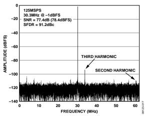
Figure 33. AD9268-125 Single-Tone FFT with  $f_{IN}$  = 30.3 MHz
