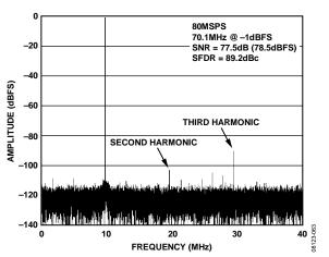
Figure 9. AD9268-80 Single-Tone FFT with  $f_{\text{IN}}$  = 70.1 MHz
