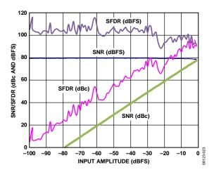
Figure 41. AD9268-125 Single-Tone SNR/SFDR vs. Input Amplitude ( $A_{\rm IN}$ ) with  $f_{\rm IN}=2.4$  MHz
