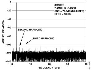
Figure 8. AD9268-80 Single-Tone FFT with  $f_{IN} = 2.4$  MHz
