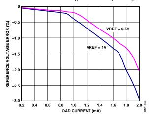
Figure 72. Reference Voltage Accuracy vs. Load Current
