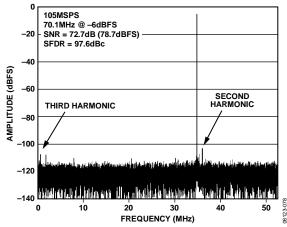
Figure 24. AD9268-105 Single-Tone FFT with  $f_{\text{IN}}$  = 70.1 MHz with Dither Enabled
