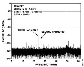
Figure 36. AD9268-125 Single-Tone FFT with  $f_{IN} = 200.3$  MHz
