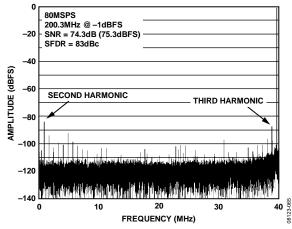
Figure 11. AD9268-80 Single-Tone FFT with  $f_{IN} = 200.1$  MHz
