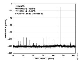
Figure 49. AD9268-125 Two-Tone FFT with  $f_{\rm IN1}$  = 169.1 MHz and  $f_{\rm IN2}$  = 172.1 MHz
