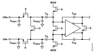
Figure 64. Switched-Capacitor Input
