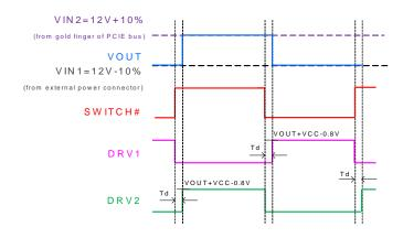
Figure 1. Fast Switching Application
