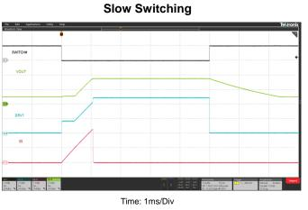
SWITCH#(2V/Div);VOUT(7V/Div);DRV1(7V/Div);DRV2(7V/Div) VIN1=12V(external path),VIN2=3.3V(internal path),IOUT=0.1A
