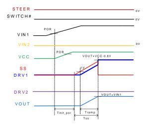
Figure 3. Power-Up Sequence of Scenario 1
