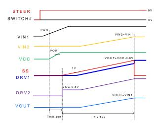
Figure 5. Power-Up Sequence of Scenario 3
