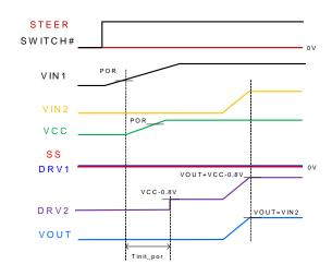
Figure 4. Power-Up Sequence of Scenario 2
