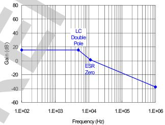
Figure 6. Frequency Response of Modulator.
