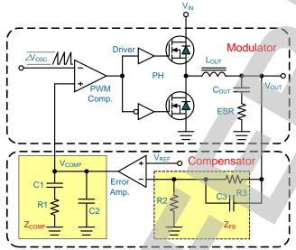
Figure 5. Voltage Control Loop Using uP1543.
