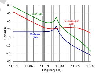
Figure 14. Frequency Response of Type III Compensation.
