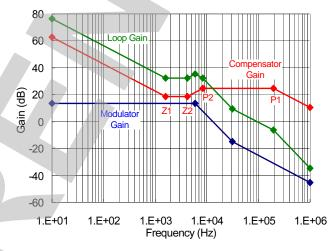
Figure 13. Loop Gain of Type III Compensation Network.
