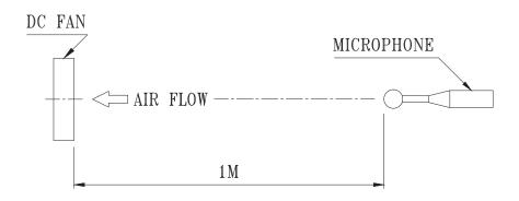
NOISE IS MEASURED AT RATED VOLTAGE IN FREE AIR IN ANECHOIC CHAMBER WITH MICROPHONE AT A DISTANCE OF ONE METER FROM THE FAN INTAKE.
