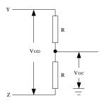
Figure 3. Driver DC Test Load
