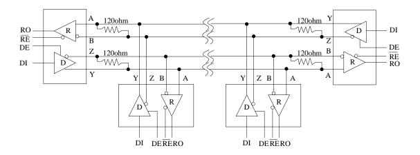
Figure 2: Typical Full-Duplex RS-422 Network
