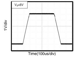
Figure 17. Large-signal Step Response
