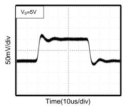
Figure 15. Small-signal Step Response
