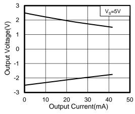
Figure 19. Output Voltage vs Output Current
