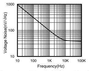
Figure 2. Input Voltage Noise Spectral Density vs Frequency
