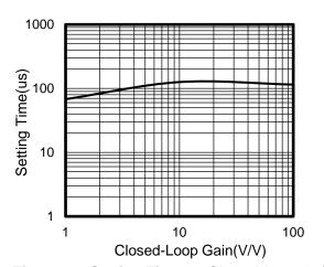
Figure 21. Setting Time vs Closed-loop Gain
