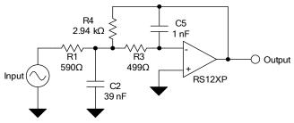
Figure 26. 25-kHz Low-Pass Filter
