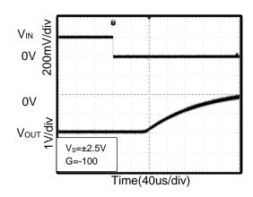
Figure 14. Negative Overload Recovery
