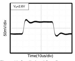
Figure 16. Small-signal Step Response
