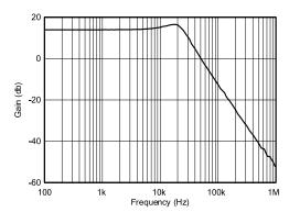
Figure 27. Low-pass filter transfer function
