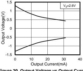
Figure 20. Output Voltage vs Output Current
