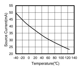
Figure 4. Source Current vs Temperature
