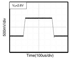
Figure 18. Large-signal Step Response
