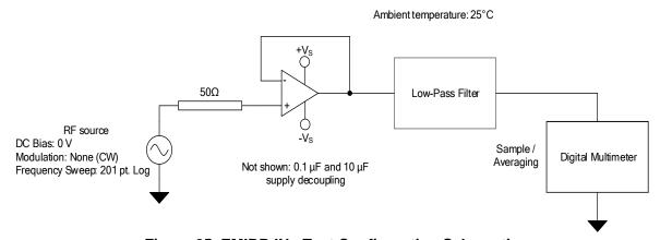
Figure 25. EMIRR IN+ Test Configuration Schematic
