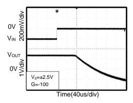
Figure 13. Positive Overload Recovery
