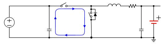
图 12-1. High Frequency Current Path
