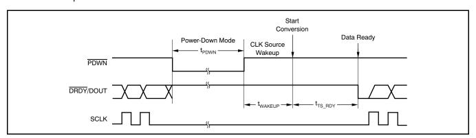
Figure 9. Wake-Up Timing from Power-Down Mode
