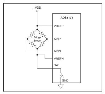
Figure 3. Low-Side Power Switch
