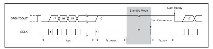
Figure 8. Standby Mode Timing (Can be used for single conversions)
