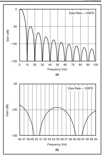
Figure 4. Nominal Frequency Response Out To 100Hz
