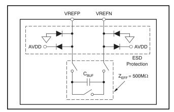
Figure 2. Simplified Reference Input Circuitry
