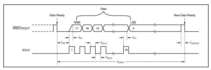
Figure 6. 18-Bit Data Retrieval Timing
