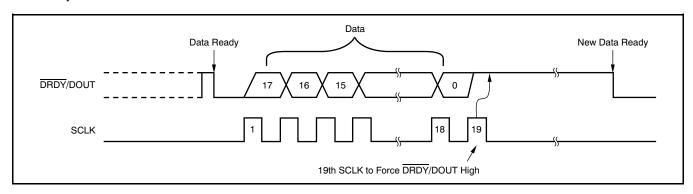
Figure 7. Data Retrieval with DRDY/DOUT Forced High Afterwards
