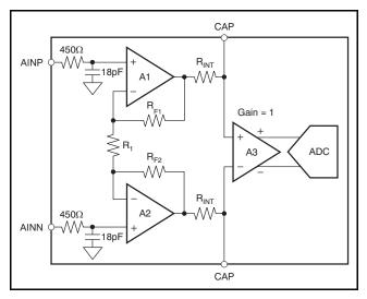
Figure 1. Simplified Diagram of the Amplifier
