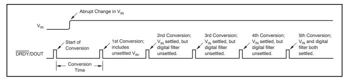
Figure 5. Settling Time in Continuous Conversion Mode
