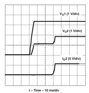
Figure 15. Prebias Startup Waveforms
