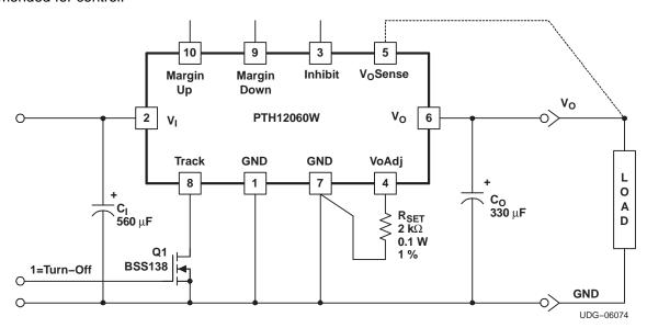
Figure 10. Basic Start-up Control Circuit
