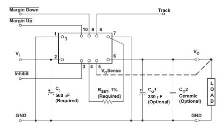
A. R<sub>SET</sub> = Required to set the output voltage to a value higher than the minimum value. See the Application Information section for values.
