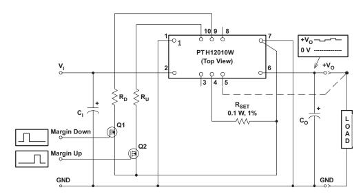
Figure 17. Margin Up/Down Application Schematic
