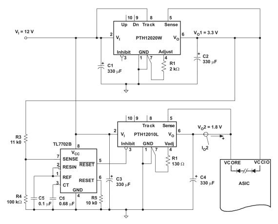
Figure 16. Application Circuit Demonstrating Prebias Startup
