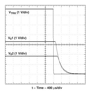
Figure 14. Simultaneous Power Down with Auto-Track Control
