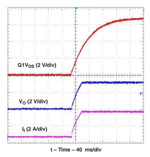
Figure 11. Power-Up from Track Control
