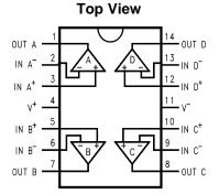
Figure 4. 14-Pin TSSOP Package See Package Number PW0014A
