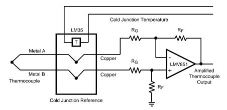
Figure 57. Thermocouple Read Out Circuit
