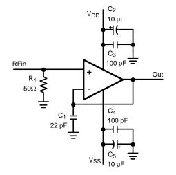
Figure 53. Circuit for Coupling the RF Signal to IN<sup>+</sup>
