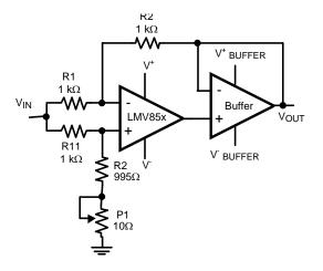
Figure 49. AC CMRR Measurement Setup
