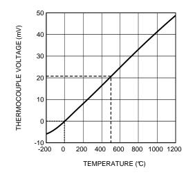
Figure 56. K-Type Thermocouple Response
