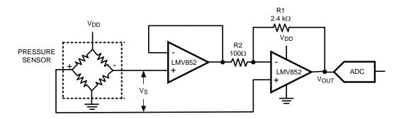
Figure 55. Pressure Sensor Application
