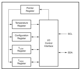
Figure 7. Internal Register Structure
