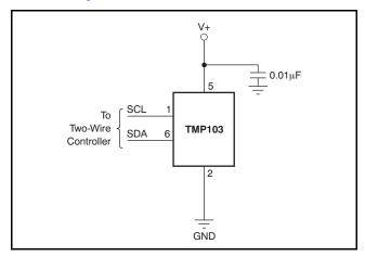
NOTE: SCL and SDA pins require pull-up resistors.
