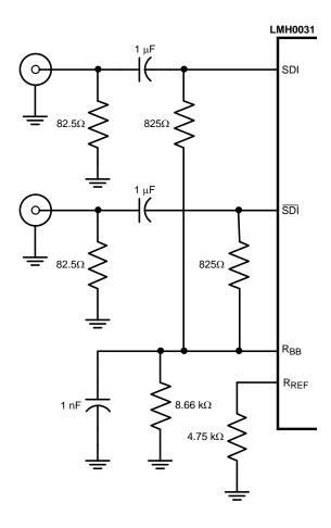
Figure 2. Optional Input Biasing Scheme
