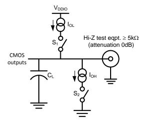
C<sub>L</sub> including probe and jig capacitance, 3pF max.
