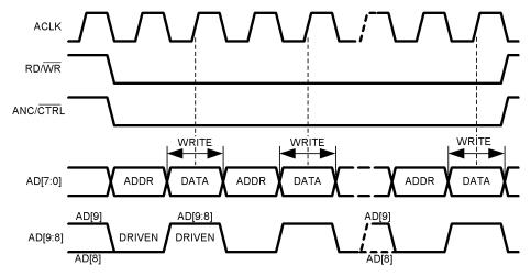
Figure 4. Control Data Write Timing
