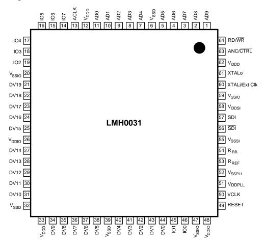
Figure 1. 64-Pin TQFP See Package Number PAG0064A
