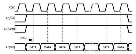
Figure 5. Ancillary Data Read Timing
