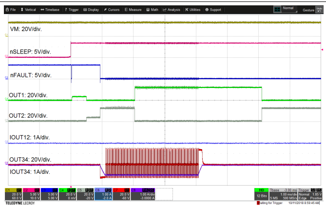
图 53. Torque Pin Functionality for Current Scaling
