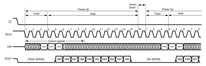
Figure 2. ADC088S102 Operational Timing Diagram
