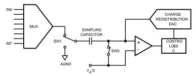
Figure 35. ADC088S102 in Track Mode
