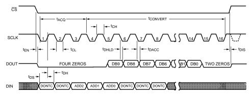
Figure 3. ADC088S102 Serial Timing Diagram
