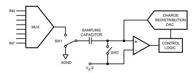
Figure 36. ADC088S102 in Hold Mode
