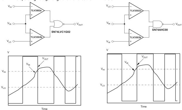
Figure 20. Window Comparator—Active High
