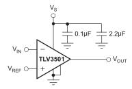
Figure 16. Basic Connections for the TLV3501
