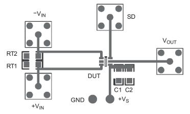
Figure 23. TLV3501DBV (SOT-23) Sample Layout
