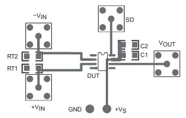
Figure 22. TLV3501D (SOIC) Sample Layout
