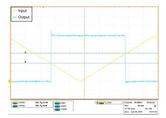
Figure 19. TLV3501 Device With Upper and Lower Thresholds With 1-V Hysteresis
