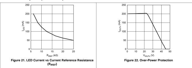
If the voltage on the IOUTn (n = 1, 2) pin is higher than 24 V when channel n is on, the regulated current of channel n reduces linearly if the voltage further increases (as shown in Figure 22). The regulated current of another channel is not affected. This over-power protection feature avoids damaging the current regulator owing to the shorting of many LEDs in one string.
