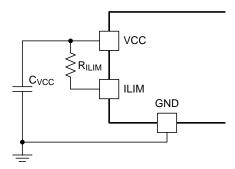
Figure 20. Programmable Current Limit
