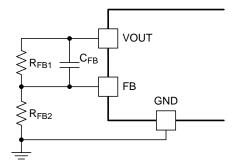
Figure 23. Output Voltage Feedback Circuit
