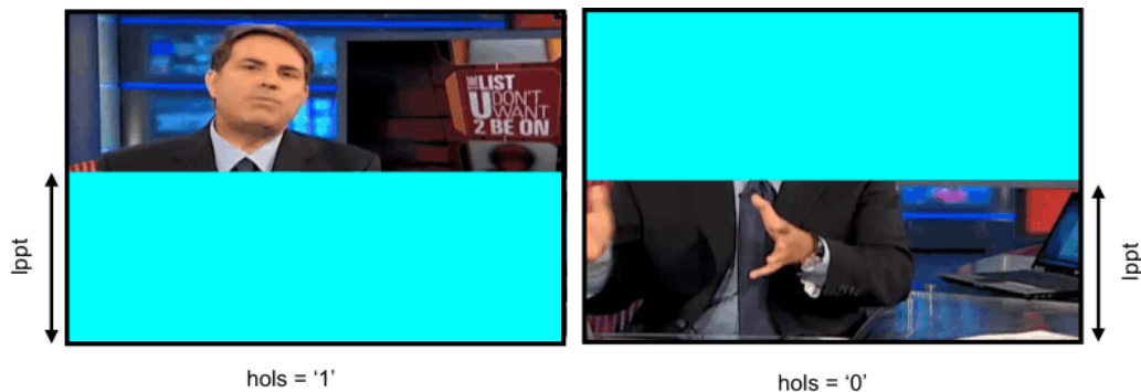
Figure 22-15. Subpicture Output with HOLS Bit Variations
