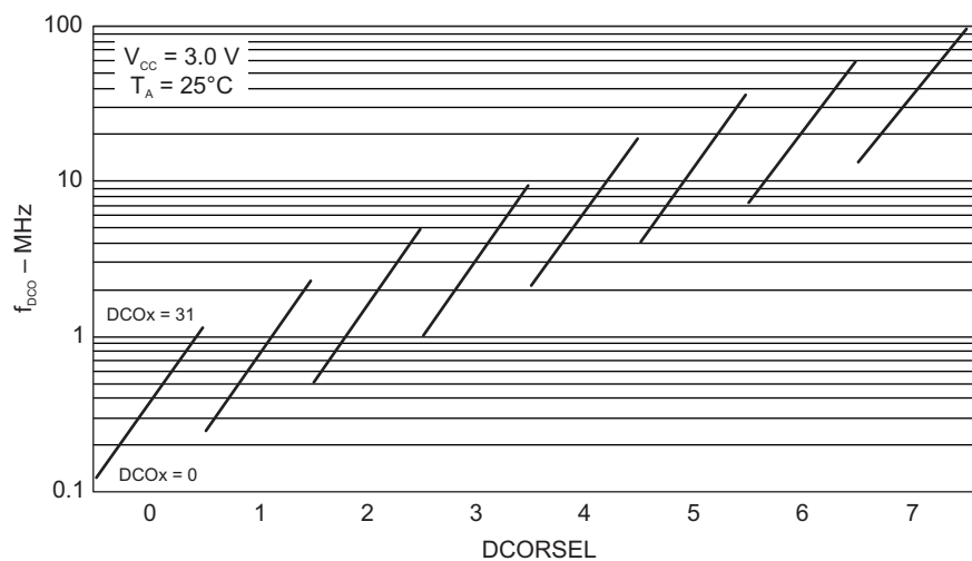
Figure 5-10. Typical DCO Frequency
