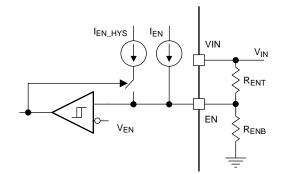
Figure 15. System UVLO By Enable Dividers
