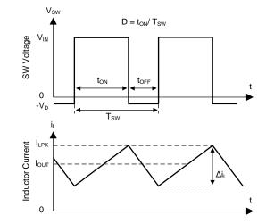
Figure 13. SW Node and Inductor Current Waveforms in Continuous Conduction Mode (CCM)
