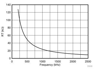
Figure 16. RT vs Frequency Curve
