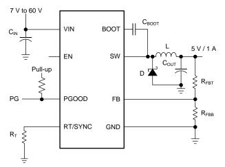
Figure 22. Application Circuit, 5V Output
