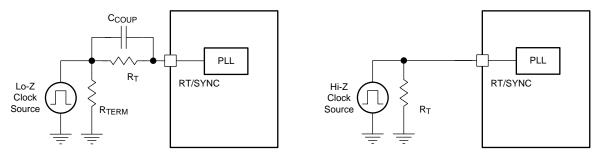
Figure 17. Synchronizing to an External Clock
