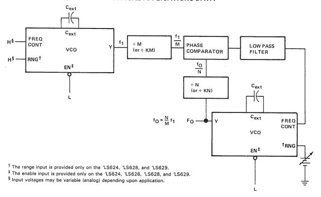
FIGURE A-PHASE-LOCKED LOOP.
