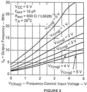
†Due to the effects of stray capacitance the output frequency may be unstable when the frequency control voltage is less than 1 volt.
