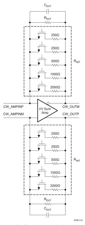
Figure 87. CW Summing Amplifier Block Diagram
