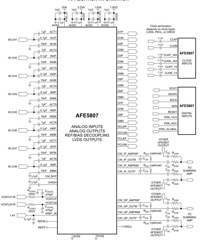
Figure 82. Application Circuit
