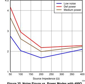
Figure 35. Noise Figure vs. Power Modes with  $400\Omega$  Termination
