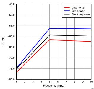
Figure 37. HD2 vs. Frequency,  $V_{\text{IN}}$  = 500 mVpp and  $V_{\text{OUT}}$  = -1dBFS
