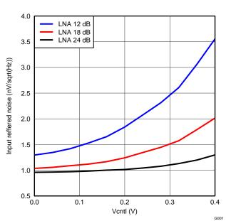
Figure 21. IRN, PGA = 24dB and Medium Power Mode
