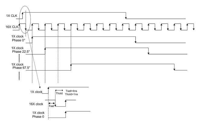
Figure 73. 1x and 16x CW Clock Timing
