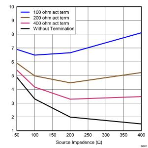
Figure 33. Noise Figure, LNA = 12dB and Low Power Mode
