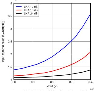
Figure 23. IRN, PGA = 24dB and Low Power Mode
