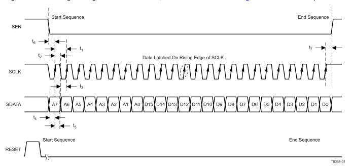
Figure 60. SPI Timing
