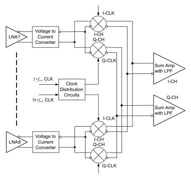
Figure 69. Simplified Block Diagram of CW Path
