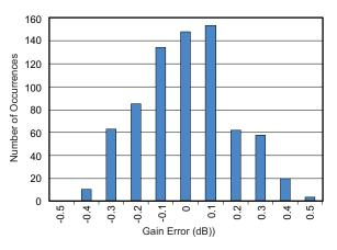
Figure 4. Gain Matching Histogram, V<sub>CNTL</sub> = 0.3V (936 Channels)
