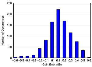
Figure 5. Gain Matching Histogram, V<sub>CNTL</sub> = 0.6V (936 Channels)
