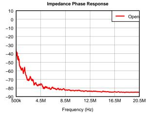
Figure 9. Input Impedance without Active Termination (Phase)
