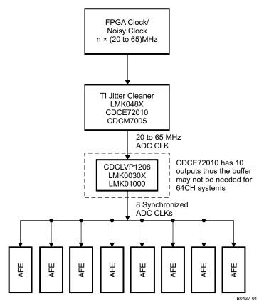
Figure 91. ADC Clock Distribution Network
