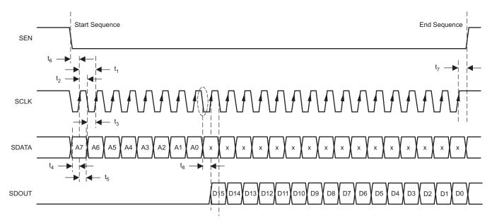
Figure 61. Serial Interface Register Read
