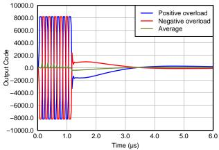
Figure 54. Pulse Inversion Asymmetrical Negative Input
