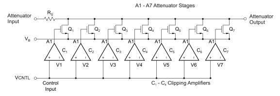
Figure 66. Simplified Voltage Controlled Attenuator (Analog Structure)
