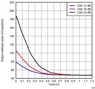
Figure 24. ORN, PGA = 24dB and Low Noise Mode
