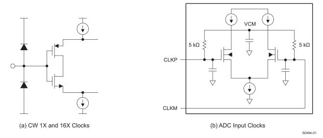
Figure 79. Equivalent Circuits of Clock Inputs
