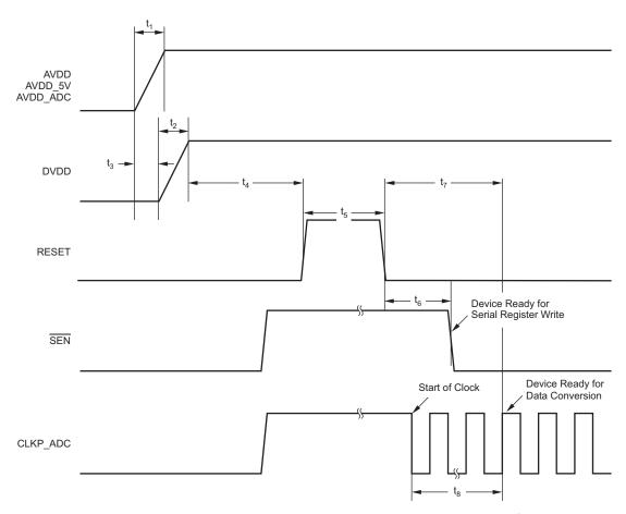
$10\mu s < t1 < 50ms$ ,  $10\mu s < t2 < 50ms$ , -10ms < t3 < 10ms, t4 > 10ms, t5 > 100ns, t6 > 100ns, t7 > 10ms, and  $t8 > 100\mu s$ . The AVDDx and DVDD power-on sequence does not matter as long as -10ms < t3 < 10ms. Similar considerations apply while shutting down the device.
