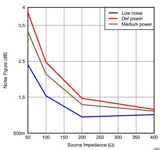
Figure 36. Noise Figure vs. Power Modes without Termination
