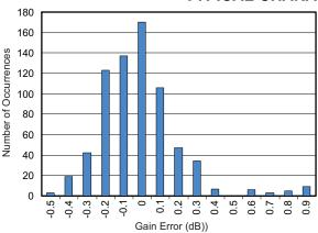
Figure 6. Gain Matching Histogram, V<sub>CNTL</sub> = 0.9V (936 Channels)
