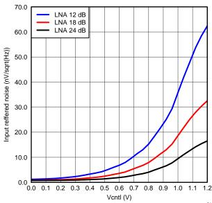
Figure 18. IRN, PGA = 24dB and Low Noise Mode
