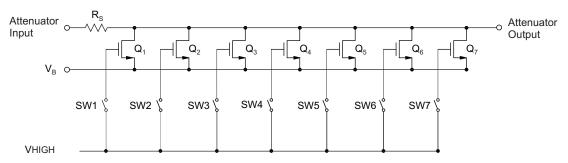
Figure 67. Simplified Voltage Controlled Attenuator (Digital Structure)
