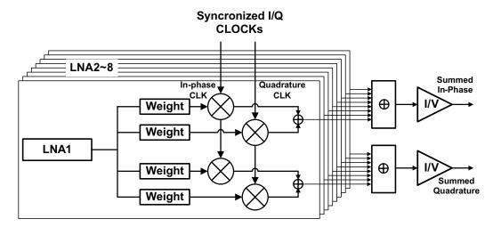
Figure 76. Block Diagram of 1 x  $f_{cw}$  mode
