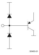
Figure 78. Equivalent Circuits of V<sub>CNTLP/M</sub>
