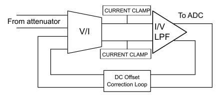
Figure 68. Simplified Block Diagram of PGA
