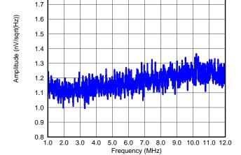
Figure 26. ORN, PGA = 24 dB and Low Power Mode
