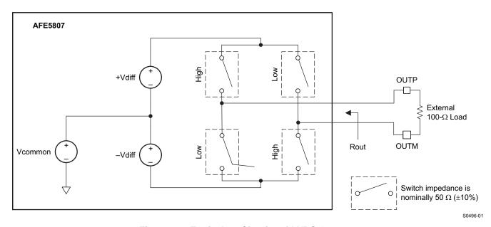
Figure 81. Equivalent Circuits of LVDS Outputs
