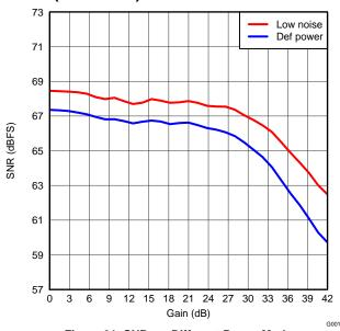
Figure 31. SNR vs. Different Power Modes
