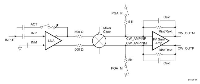
Figure 92. AFE5807 PGA Test Mode
