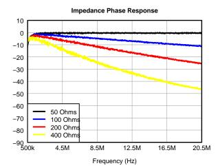
Figure 11. Input Impedance with Active Termination (Phase)
