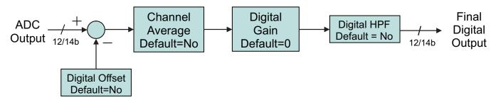
Figure 63. ADC Digital Block Diagram
