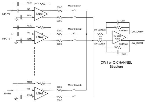
Note: the 10~15  $\Omega$  parasitic resistors at CW\_AMPINM/P are due to internal IC routing and can create slight attenuation.
