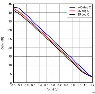
Figure 3. Gain Variation vs. Temperature, LNA = 18dB and PGA = 24dB
