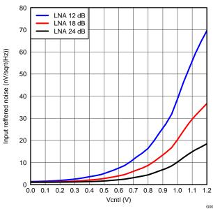
Figure 22. IRN, PGA = 24dB and Low Power Mode
