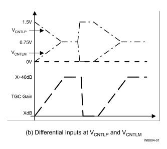
Figure 86. V<sub>CNTLP</sub> and V<sub>CNTLM</sub> Configurations
