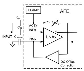
Figure 65. AFE5807 LNA with DC Offset Correction Circuit
