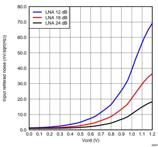
Figure 20. IRN, PGA = 24dB and Medium Power Mode
