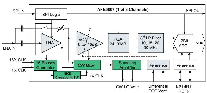
Figure 64. Functional Block Diagram
