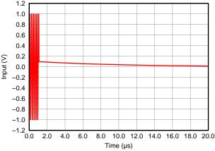
Figure 52. V<sub>CNTL</sub> Response Time, LNA = 18dB and PGA = 24dB
