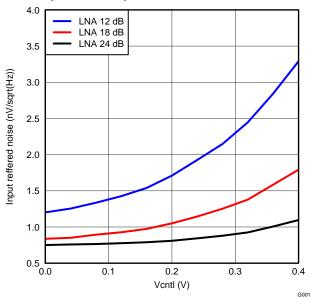
Figure 19. IRN, PGA = 24dB and Low Noise Mode
