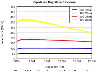
Figure 10. Input Impedance with Active Termination (Magnitude)
