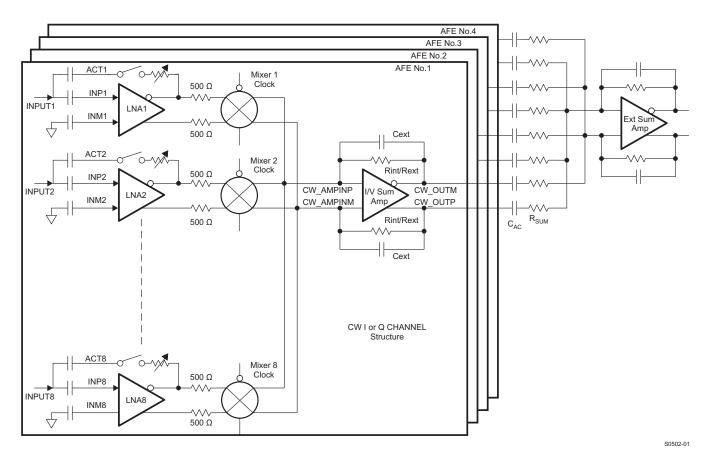
Figure 88. CW circuit with Multiple AFE5807s
