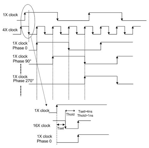
Figure 75. 8 x  $f_{cw}$  and 4 x  $f_{cw}$  Timing Diagram
