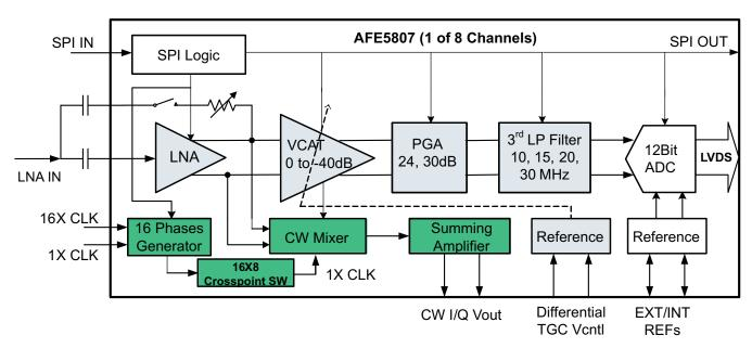
Figure 1. Block Diagram
