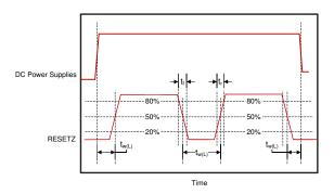
图 6-6. Power-Up and Power-Down RESETZ Timing
