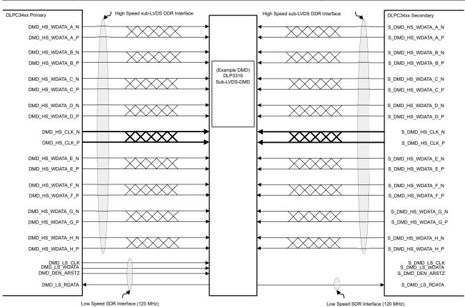
图 7-12. DLP3310 (.33 1080p) DMD Interface Example (Option 1 and 2)
