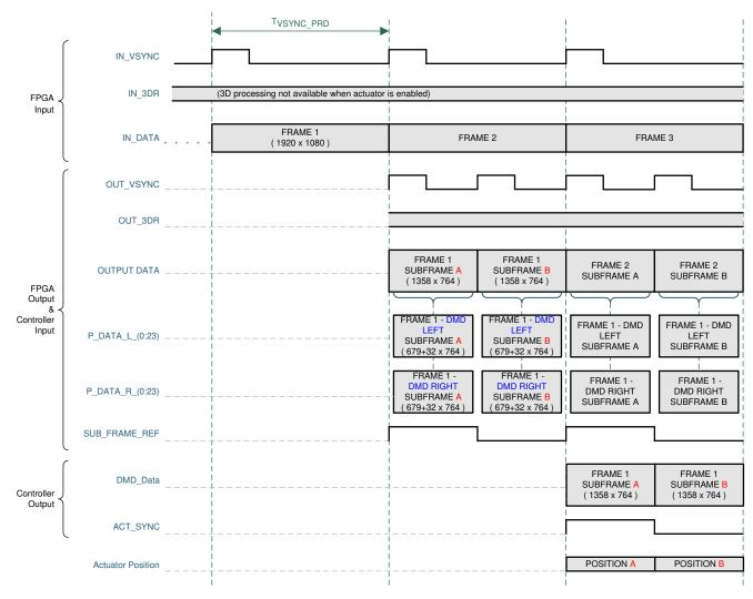
图 7-2. DLPC3437 2D Actuator Frame and Signal Timing
