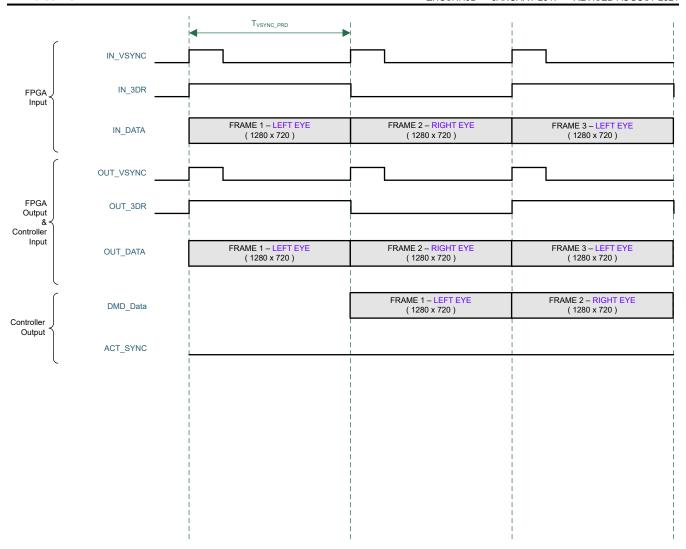
图 7-3. DLPC3437 3D Frame and Signal Timing
