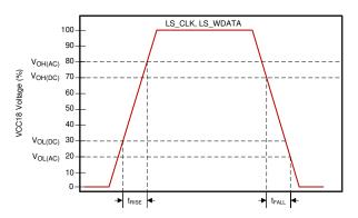
图 6-3. LS\_CLK and LS\_WDATA Slew Rate
