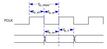
图 6-8. Parallel Interface General Timing
