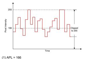
图 7-6. Source Pixels for a Color Channel
