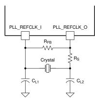
$$\begin{split} &C_L = Crystal \ load \ capacitance \ (farads) \\ &C_{L1} = 2 \times (C_L \ - \ Cstray\_pll\_refclk\_i) \\ &C_{L2} = 2 \times (C_L \ - \ Cstray\_pll\_refclk\_o) \end{split}$$
