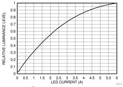
图 8-2. Typical Luminance vs Current
