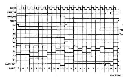
Fig. 16 — Timing diagram for CD4516B.
