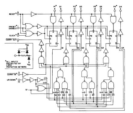
Fig. 10 - Logic Diagram for CD4516B.
