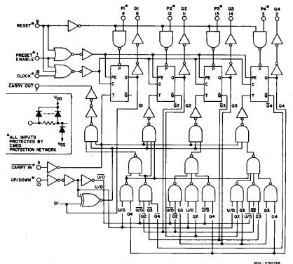
Fig.3 — Logic Diagram for CD45108.
