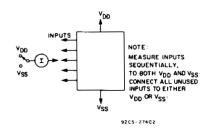
Fig. 12 - Input-current test circuit.
