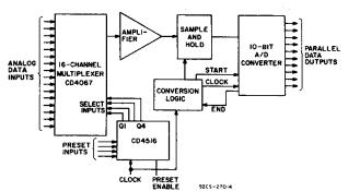
This acquisition system can be operated in the random access mode by jamming in the channel number at the present inputs, or in the sequential mode by clocking the CD4516B.
