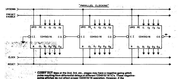
\* CARRY OUT lines at the 2nd, 3rd, etc., stages may have a negative-going glitch pulse resulting from differential delays of different CD4510/16 IC's. These negative-going glitches do not affect proper CD4510/16 operation. However, if the CARRY OUT signals are used to trigger other edge-sensitive logic devices, such as FF's or counters, the CARRY OUT signals should be gated with the clock signal using a 2-input OR gate such as CD4071B.
