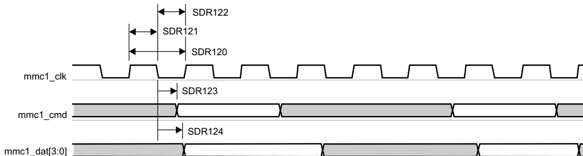
Figure 5-81. MMC/SD/SDIO in - High Speed SDR12 - Transmitter Mode
