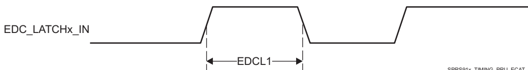
Figure 5-119. PRU-ICSS ECAT LATCHx_IN Timing
