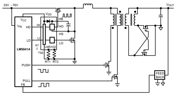
Figure 1. Simplified Cascaded Push-Pull Power Converter
