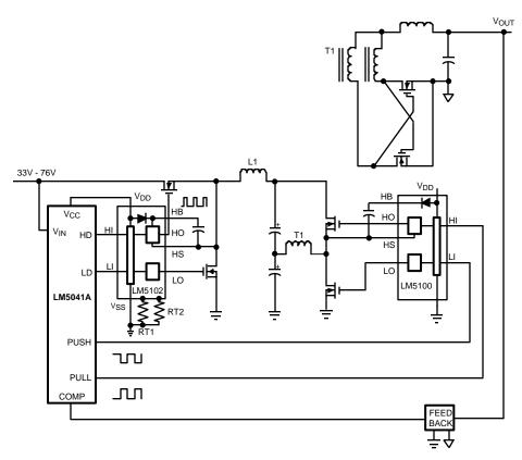
Figure 14. Simplified Cascaded Half-Bridge
