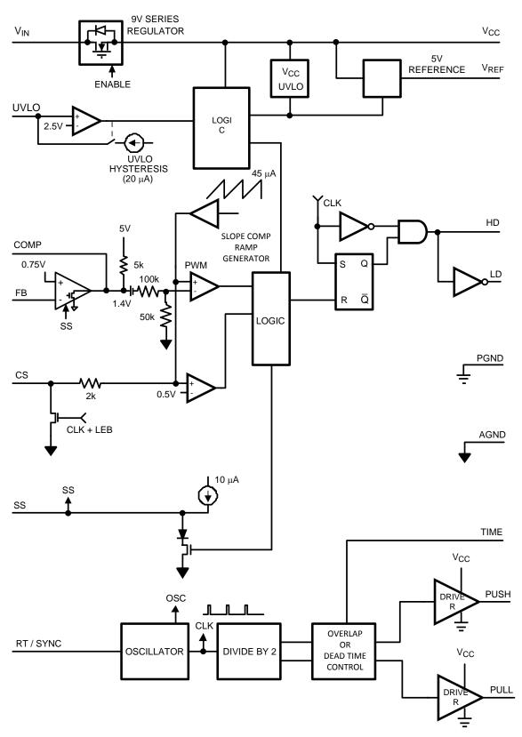
Figure 3. Simplified Block Diagram
