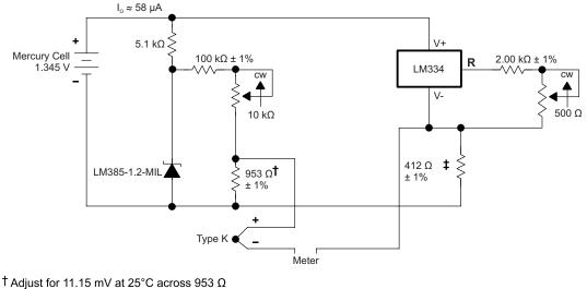
I Adjust for 11.15 mV at 25°C across 953  $\Omega$ ‡ Adjust for 12.17 mV at 25°C across 412  $\Omega$
