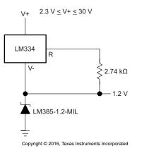
Figure 11. Generating Reference Voltage With a Constant Current Source Device
