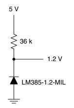
Figure 8. Generating Reference Voltage With a Resistive Current Source
