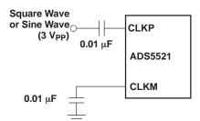
Figure 46. AC-Coupled, Single-Ended Clock Input
