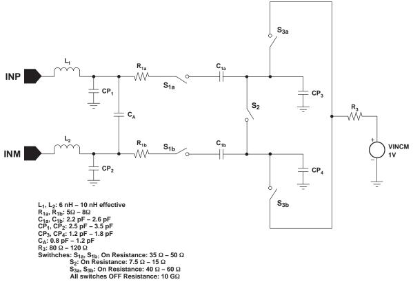
A. All Switches are ON in sampling phase which is approximately one half of a clock period.
