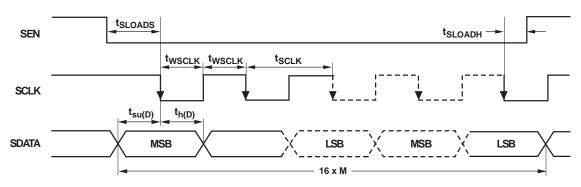
Figure 4. Serial Programming Interface Timing Diagram
