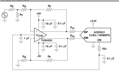
Figure 42. Using the THS4503 with the ADS5521
