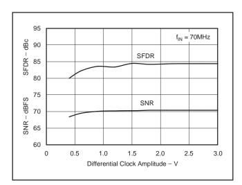
Figure 49. AC Performance vs Clock Amplitude
