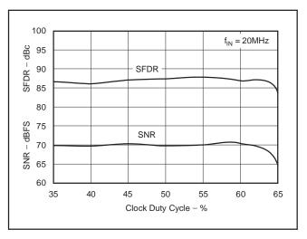
Figure 48. AC Performance vs Clock Duty Cycle
