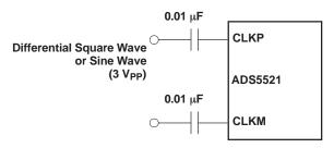
Figure 47. AC-Coupled, Differential Clock Input
