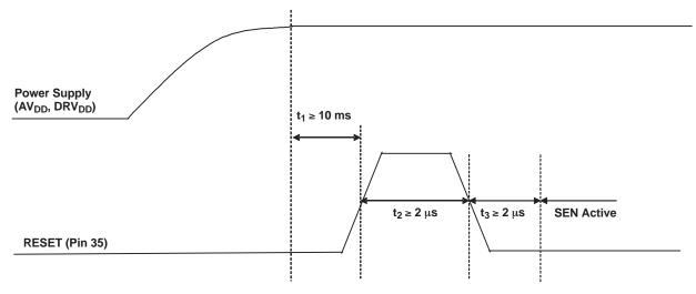
Figure 2. Reset Timing Diagram
