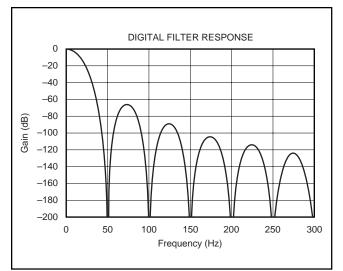
FIGURE 4. Digital Filter Response (50Hz).
