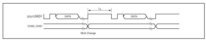
FIGURE 12. Multiplexer Operation.
