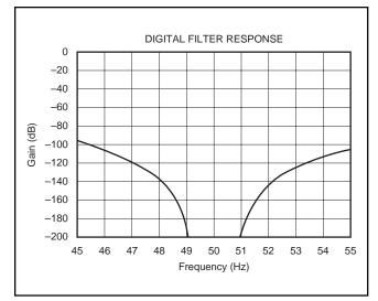
FIGURE 7. Expanded Digital Filter Response (50Hz with a 50Hz data output rate).
