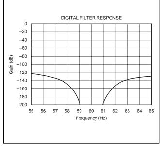
FIGURE 10. Expanded Digital Filter Response (60Hz with a 10Hz data output rate).
