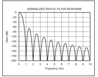
FIGURE 3. Normalized Digital Filter Response.
