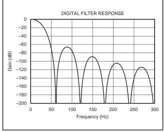
FIGURE 5. Digital Filter Response (60Hz).
