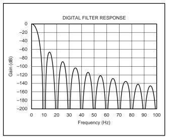
FIGURE 6. Digital Filter Response (10Hz).
