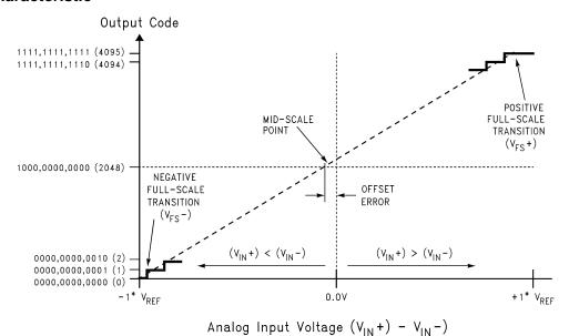
Figure 2. Transfer Characteristic
