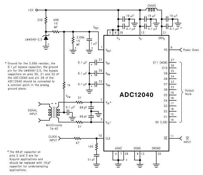
Figure 23. Driving the Signal Inputs with a Transformer
