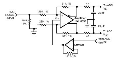
Figure 22. Differential Drive Circuit of Figure 21
