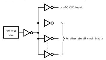
Figure 25. Isolating the ADC Clock from other Circuitry with a Clock Tree
