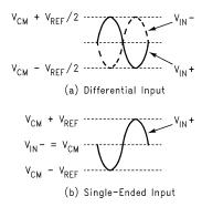
Figure 19. Expected Input Signal Range
