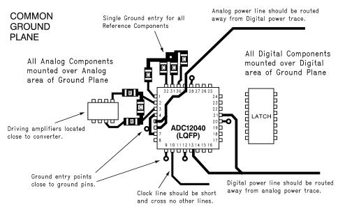
Figure 24. Example of a Suitable Layout
