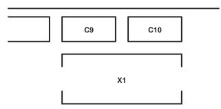
Figure 11. Recommended Crystal and Capacitor Layout
