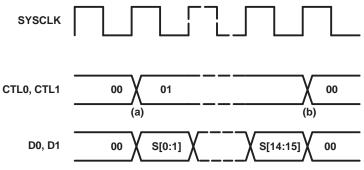
Figure 14. Status Transfer Timing
