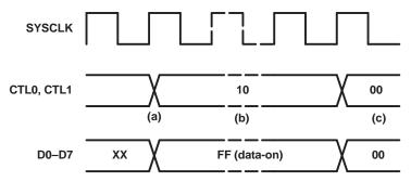
Figure 16. Null Packet Reception Timing
