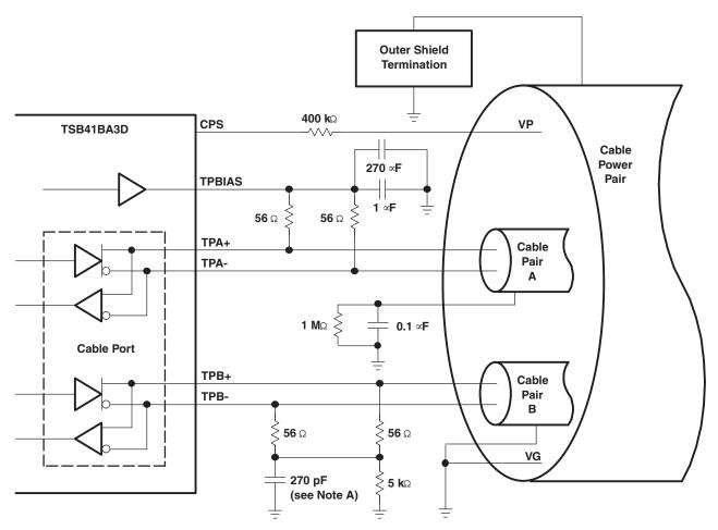
A. The IEEE Std 1394-1995 calls for a 250-pF capacitor, which is a nonstandard component value. A 270-pF capacitor is recommended.
