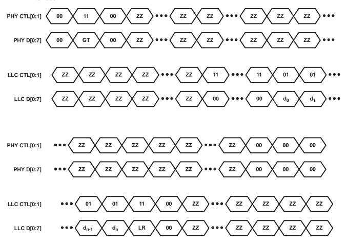
Figure 29. Transmit Packet Timing With Optional Link Request
