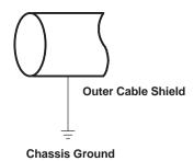
Figure 6. Non-DC-Isolated Outer Shield Termination
