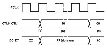
Figure 28. Null Packet Reception Timing
