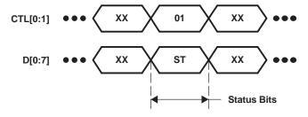
Figure 24. Bus Status Transfer Timing
