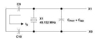
Figure 10. Load Capacitance for the TSB41BA3D PHY
