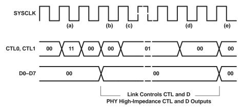
Figure 18. Cancelled/Null Packet Transmission
