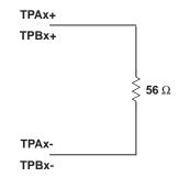
Figure 1. Test Load Diagram
