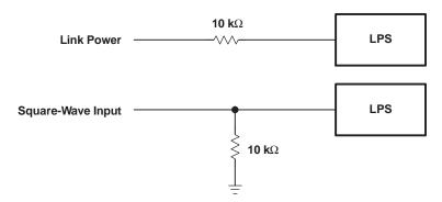
Figure 7. Nonisolated Connection Variations for LPS
