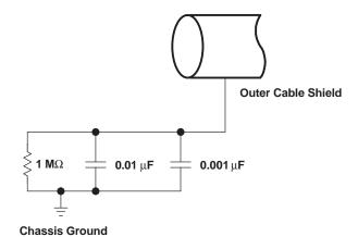
Figure 5. Typical DC-Isolated Outer Shield Termination
