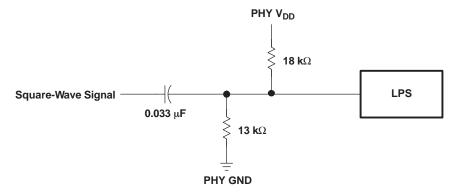
Figure 8. Isolated Circuit Connection for LPS
