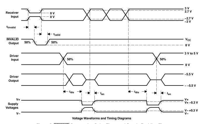
Figure 5. INVALID Propagation-Delay Times and Supply-Enabling Time
