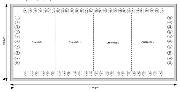
Figure 28. Device Dimensions and Pad Locations
