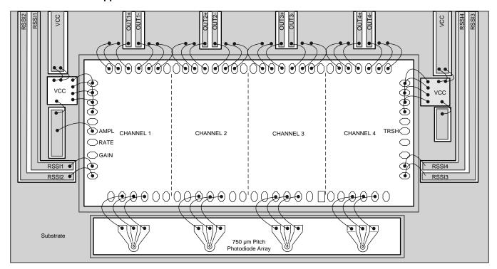
Figure 24. Basic Application Circuit with Pad Control
