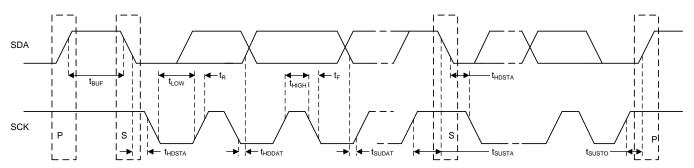
Figure 13. I<sup>2</sup>C Timing Diagram
