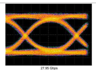
Figure 10. Output Eye-Diagram, 500-µA<sub>PP</sub> Input Current
