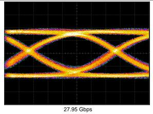
Figure 11. Output Eye-Diagram, 1.5-mA<sub>PP</sub> Input Current
