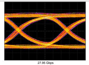
Figure 12. Output Eye-Diagram, 2.5-mA<sub>PP</sub> Input Current
