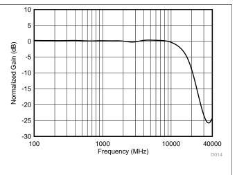
Figure 25. Gain vs Frequency (Without De-Embedding)
