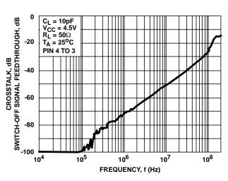
FIGURE 3. SWITCH-OFF SIGNAL FEEDTHROUGH AND CROSSTALK vs FREQUENCY,  $V_{CC}$  = 4.5V
