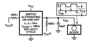
FIGURE 7. CONTROL-TO-SWITCH FEEDTHROUGH NOISE TEST CIRCUIT
