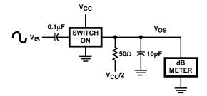
FIGURE 5. FREQUENCY RESPONSE TEST CIRCUIT
