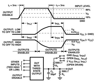
†FOR AC SERIES ONLY: WHEN V $_{\text{CC}}$  = 1.5V,  $\text{R}_{\text{L}}$  = 1k $\Omega$
