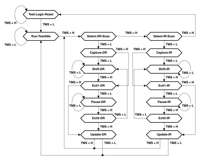
Figure 1. TAP-Controller State Diagram
