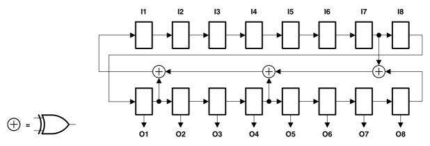
Figure 5. 16-Bit PRPG Configuration
