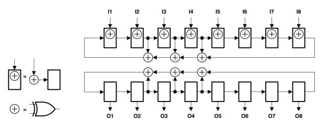
Figure 7. 8-Bit PSA/PRPG Configuration
