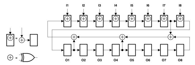
Figure 6. 16-Bit PSA Configuration
