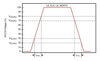
图 6-3. LS\_CLK and LS\_WDATA Slew Rate
