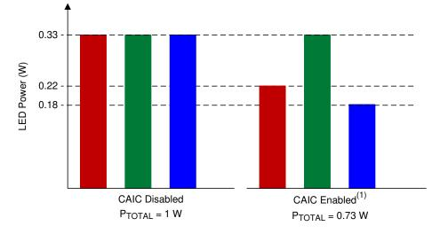
(1) With CAIC enabled, if red and blue LEDs require less than nominal power for a given input image, the red and blue LED power will reduce.
