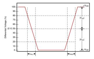
V<sub>CM</sub> is removed when the signals are viewed differentially. 图 6-2. Differential Output Signal
