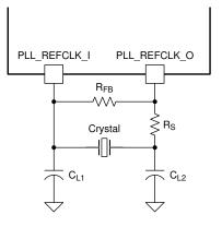
$C_L$  = Crystal load capacitance (farads)
