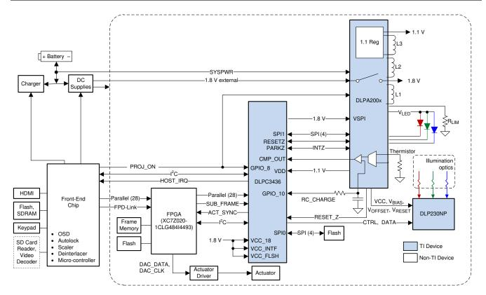
图 8-1. Typical Application Diagram (using DLPA200x)
